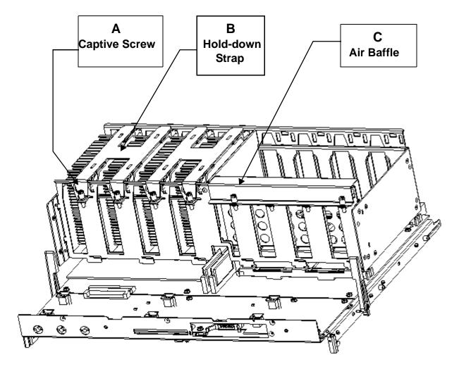
Figure 2-7: Processor Retention Mechanism
